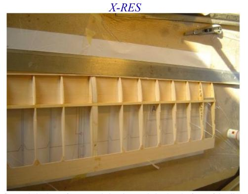
Now a strip of 2 mm balsa is cut from scrap balsa sheet and glued to the front of the ribs. Take a long sanding block to make the front edge straight.
