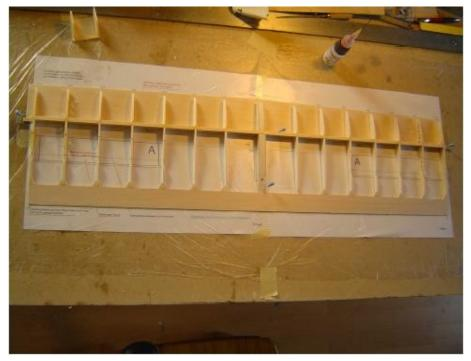
Thereafter, the middle part can be taken from the Plan and the bottom sheeting can be fully glued to the ribs.
