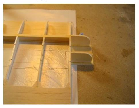
Roughen and thoroughly clean aluminum wing joiner tubes. Slide aluminum tube into ribs A-9 and A-8. Align at 90° to end rib. Gap between tube and spar webbing should be filled in with scrap 1.5mm plywood. Coat ply filler, Al tube, and spar webs with epoxy and assemble. Picture shows top spar in place, but do this step before top spar is glued in so the ply filler can be inserted.
