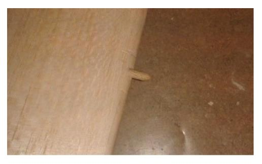
When wing is lined up, glue the ply wing locating piece in the fuselage. Remove the wing and reinforce glue the wing retaining piece in the fuselage.
