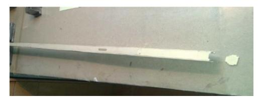
Finally, the adjustable tow hook and the balsa nose are glued with white glue. To accommodate trim weight, the nose can be slightly hollowed.
