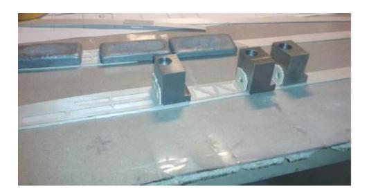
Glue the fuse bulkheads with superglue. Make sure that these are perpendicular to the fuse sides. Now two 4x4mm balsa longerons are glued in place on each fuselage side. Up to the wing saddle (bulkhead 5) on top and to the nose on the bottom.
