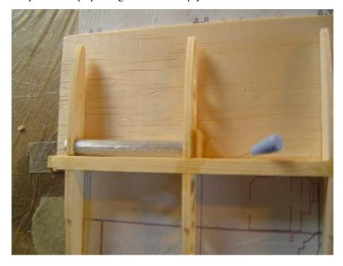
Glue in the top spar using plenty of glue. Carefully remove assembly from building board and turn over. Fit and glue on the trailing edge balsa, flush with the top of the ribs, gluing from the bottom side.
