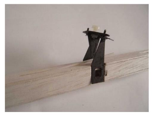
Glue the elevator mounting plates to the fuse sides, making sure the horizontal elevator plate is parallel and level with the wing. Cut the pushrod housing to length.
