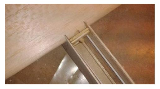
The wing retaining piece in the fuselage.
