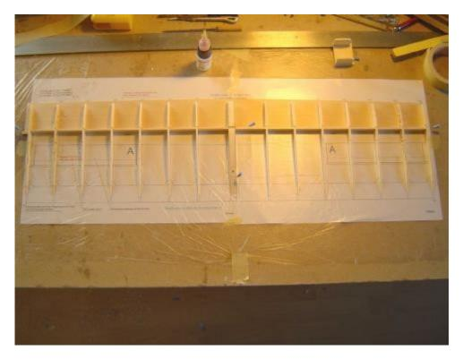
Aligning end rib A9 with 5  $^{\circ}$  angle jig.
