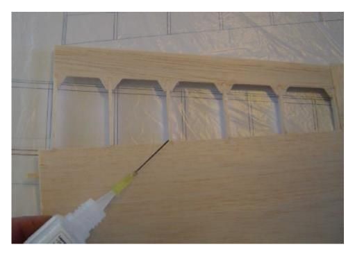
Sand front edge of outer wing flat and glue on 4x10 mm leading edge. Sand leading edge to shape using the plywood templates. They are marked with the rib locations they correspond to.
