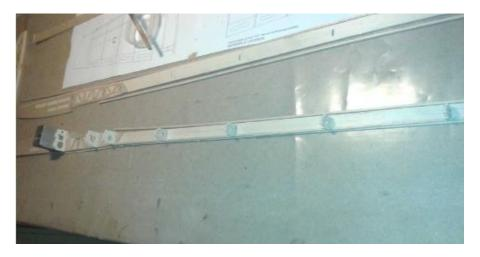
Use a spacer with 2 mm offset to locate the longerons.
