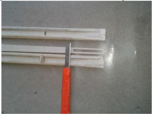
Now the pushrod housings are sanded with rough sandpaper and run through the bulkheads, but not glued.
