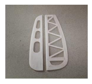
The elevator is sanded to the same airfoil shape as the rudder.
