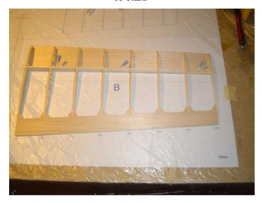
Fit the aluminum wing joiner tubes and check alignment for each mid span wing to the center wing. The exact angle is not critical, they just need to be the same for each side. When adjusted, glue in place with epoxy. Shim the gap between the tube and the spar webs with scrap ply. Fit and glue the upper spar cap, align shear webs and spar caps. Remove
