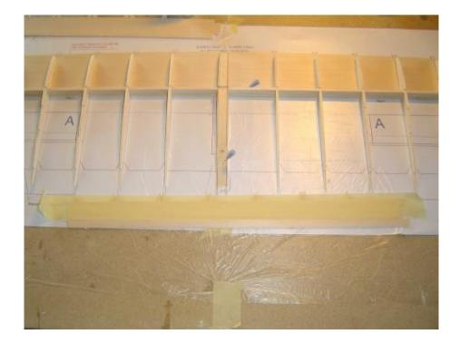
The wing can be turned right side up and the trailing edge can be sanded to a taper on the top side, starting from about 12 mm from the edge, so it is about 1mm thick at the trailing edge. Masking tape can be used to protect the area that is not sanded.
