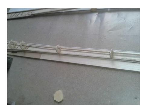
Next, the fuselage sides are glued together. Make sure they are parallel.
