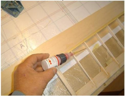
Now, through the gap between the strip on the nose and the upper sheeting, glue the upper sheeting to the ribs. Here it is advisable to use thin needles and take advantage of the fluidity of the superglue. Sheeting through the gap from the front are glued to the ribs.
