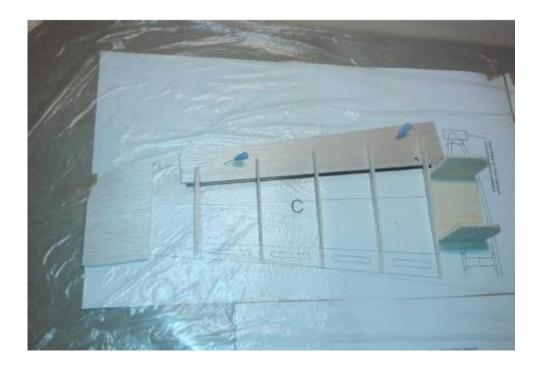
Make a false leading edge from 2mm scrap balsa. Shape top edge for upper sheeting. Cut top sheeting so it will extend over the wing tip. Glue on upper sheeting.
