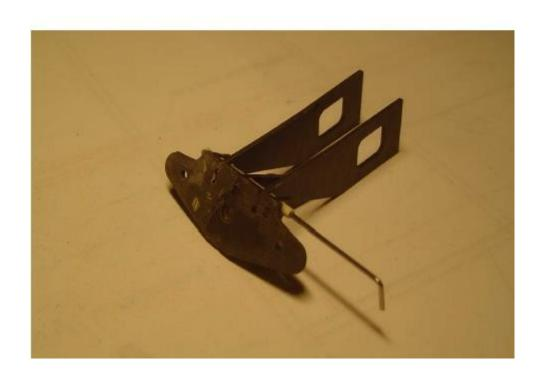
The elevator pivot is located in front of the last bulkhead. Notch the fuse sides for the elevator mounting side plates. Install the horizontal elevator plate onto the side plates using a piece of wire.
